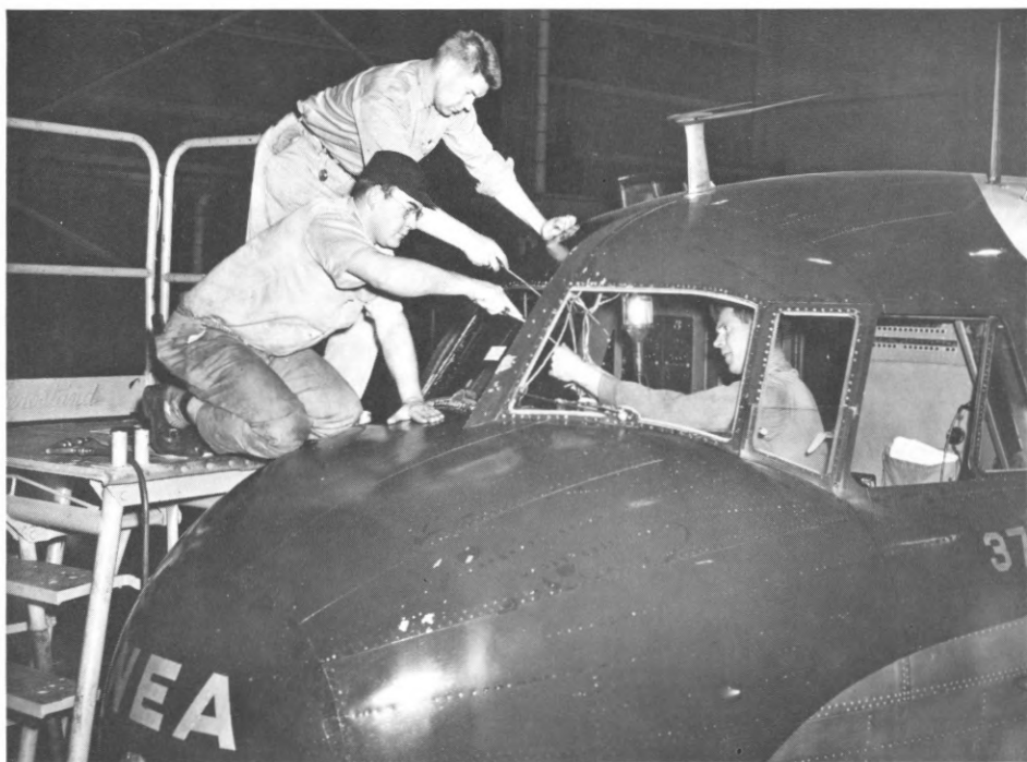
Mechanics Ed Runge, Dick Grahn and Nelson Wentworth (left to right) were replacing front windshield of a Convair 240.
