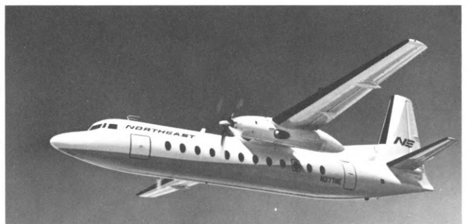
Also in 1966 the 44-passenger, 220-m.p.h. Fairchild Hiller FH-227s were put into service in the smaller New England markets.
