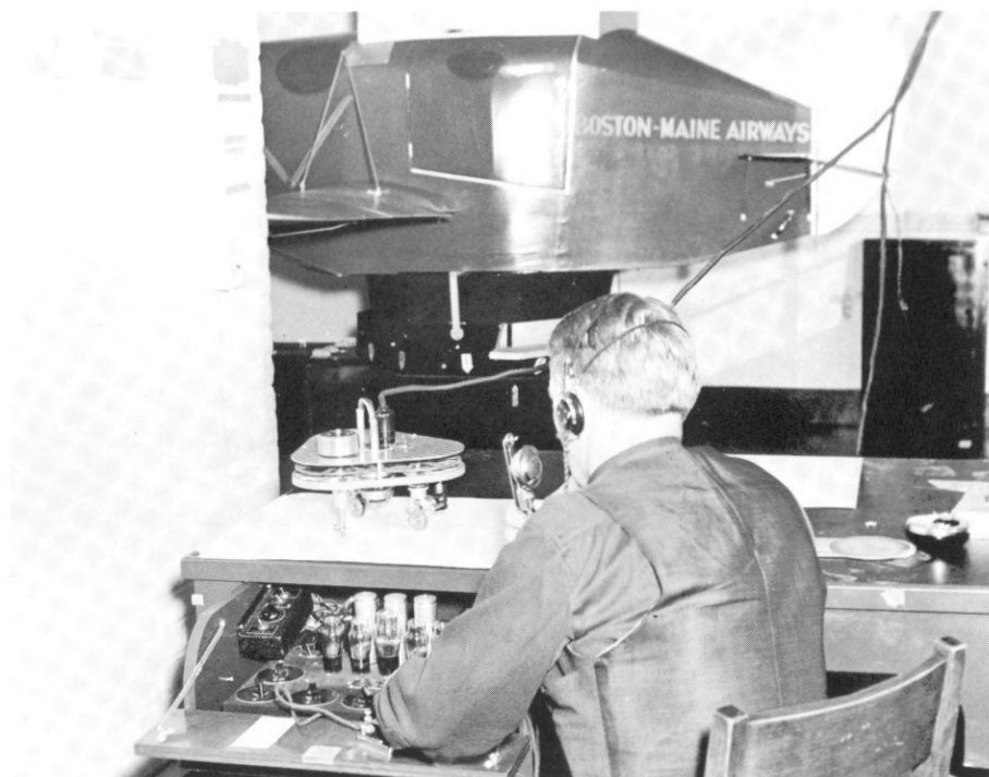
In the late 30s and early 40s NE (known as B&M Airways until November, 1940) set up one of the industry's first training departments, which included the link trainer pictured here.
