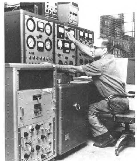
Harry Haroutunian tried out a new A.C. generator and constant speed drive test stand.
