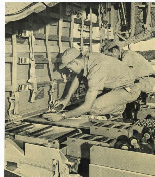
T-shaped locking bars swing up into place from the floor of the Hercules to secure pallets firmly in place. Manually inserted pins hold locking bars tight against pallets.
