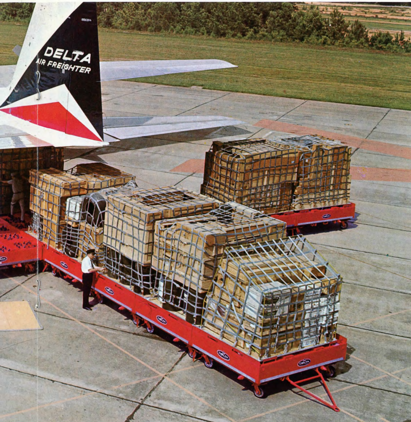
Palletized shipments roll easily through the 9' x 10' rear door into the Hercules 3,409 cu. ft. cargo compartment, then glide forward along floor-mounted roller tracks.
