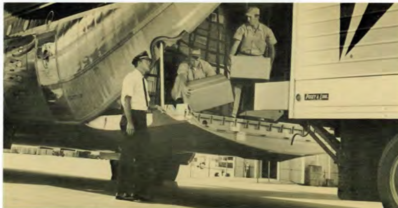
Hercules loading ramp can be adjusted from ground level to truck bed height, forming a bridge for quick and easy transfer of all types of cargo.
