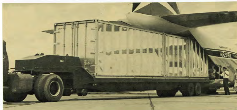
Delta's Hercules supplies the missing link for freight movements involving rail, ship, highway and air transport. In the picture above, three freight containers—two of 8' x 8' x 10' size and one 8' x 8' x 20'—are transferred directly from trailer truck to Hercules.
