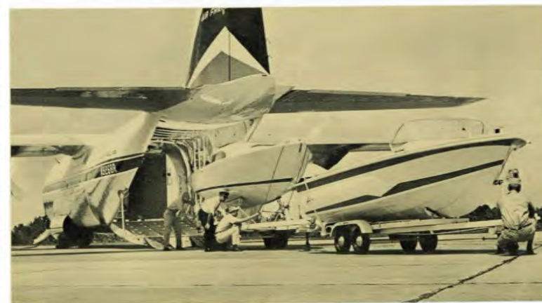
Outsize loads are no problem. The sailboat is 24' long, has a 7'10" beam, is 7' high. The motorboat nested under the bigger craft is 18' long, 7'5" wide.
